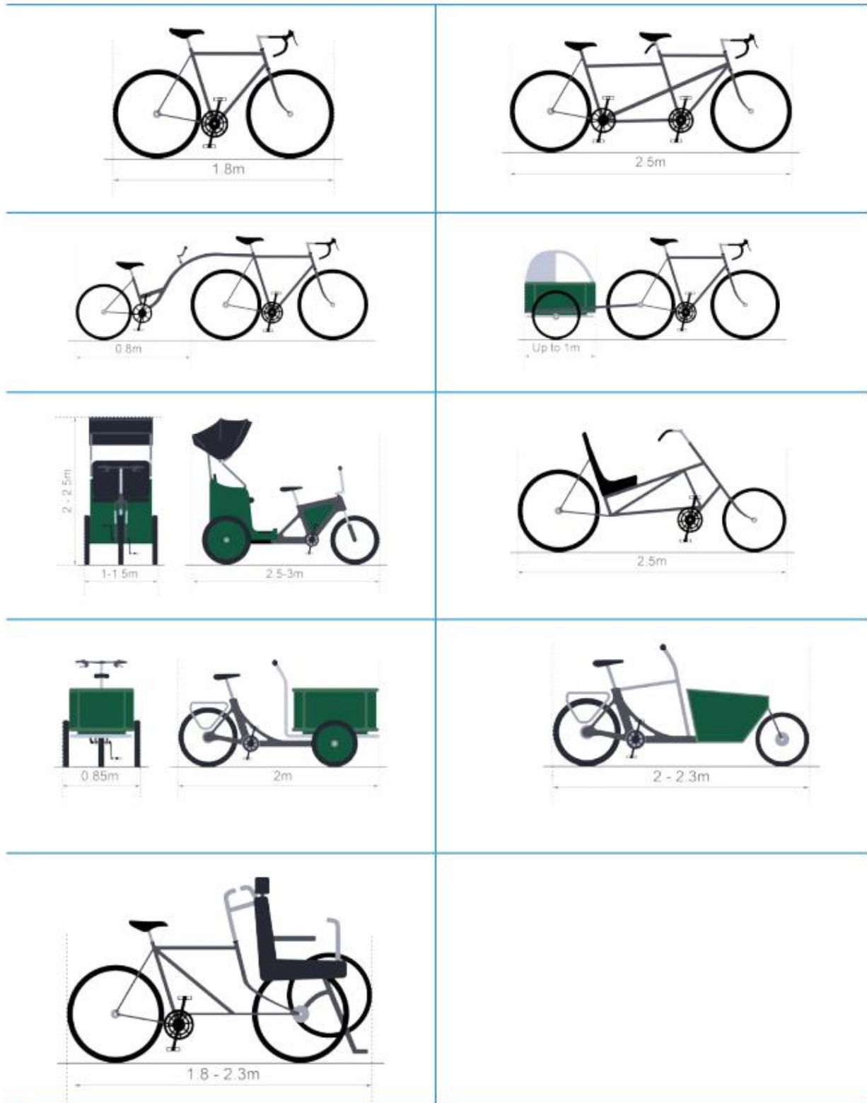
Figure 3 - Typical forms of cycles and their dimensions
